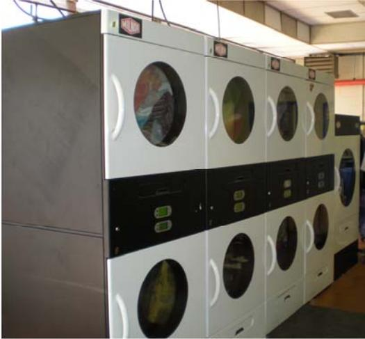
gas dryers (170 lb. capacity each). Also, the laundry boasts eight Milnor M3131 stack dryers and one M50SL steam dryer used for the residents' personal clothing.
