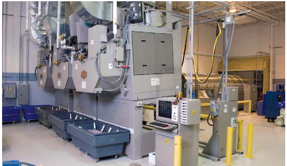
After studying its production goals and the linen demands of its hospital customers, CDHL, with guidance from The Minnesota Chemical Co., chose to replace a "mint condition" tunnel with this eight-module, 110-pound-capacity CBW tunnel washing system, including a single-stage press and three pass-through dryers.
