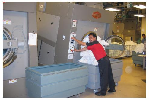
LWS45 Top Load Speed Queen Washer and a LES37 Speed Queen small electric dryer in use. The laundry uses a custom Heat Recovery System from Thermal Engineering.
