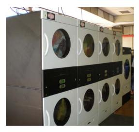
gas dryers (170 lb. capacity each). Also, the laundry boasts eight Milnor M3131 stack dryers and one M50SL steam dryer used for the residents' personal clothing.
